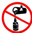
**Never** pour the mixed material into the containers with a shape narrowing towards the outlet
